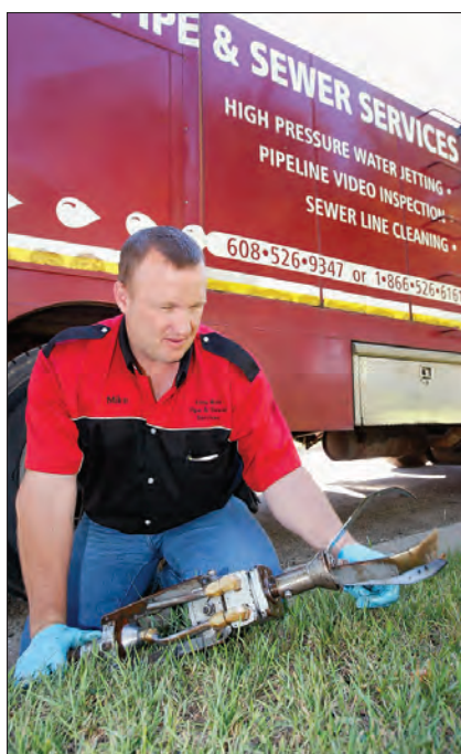
Flow-Rite owner Mike Happel prepares to launch a SRECO-FLEXIBLE root saw.
